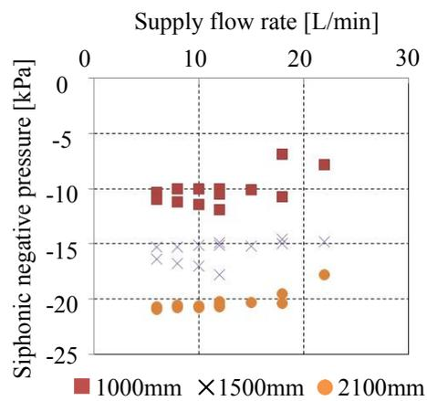
**Figure 9 Siphonic negative pressure and supply flow rate summarized by outflow head**
