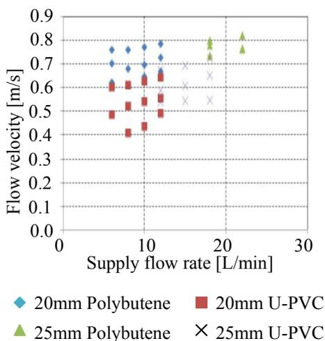
**Figure 10 Flow velocity and supply flow rate summarized by pipe material and diameter**
