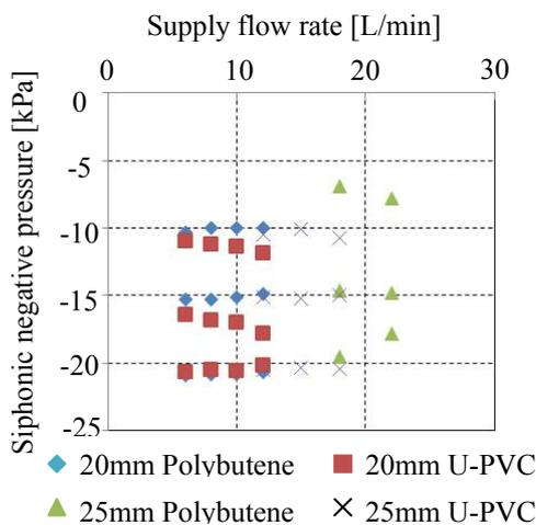
**Figure 8 Siphonic negative pressure and supply flow rate summarized by pipe material and diameter**
