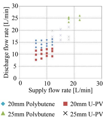
**Figure 11 Discharge flow rate and supply flow rate summarized by pipe material and diameter**
